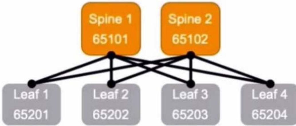
For a fully configured and functional IP fabric underlay as shown in the exhibit, how many external BGP neighbors are expected to be in the established state for Spine 1?
